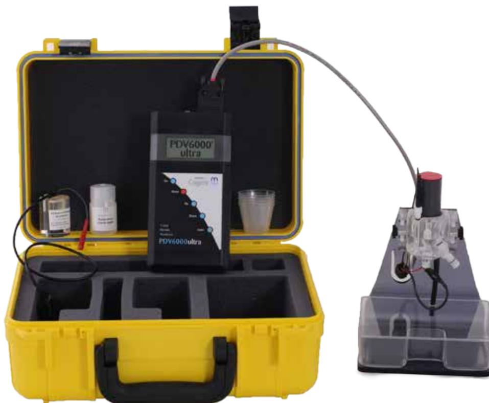
The PDV6000ultra has been upgraded to allow much improved stand-alone operation and an indication of blank and standard run performance. A larger screen allows simple voltammograms to be shown. The USB connector replaces the serial port. The upgraded product has a battery life indicator and can be run either on 4 x 1.5V AA batteries, or from the mains using the standard 8 - 12V DC transformer.
